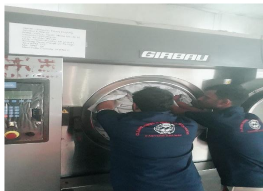
Loading of linen in washer cum extractor
