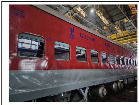
Newly PU painted coach exterior with Anti-Graffiti coating
