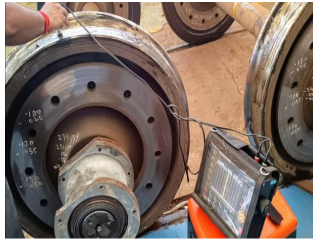
Ultrasonic Scanning of Tread Portion
