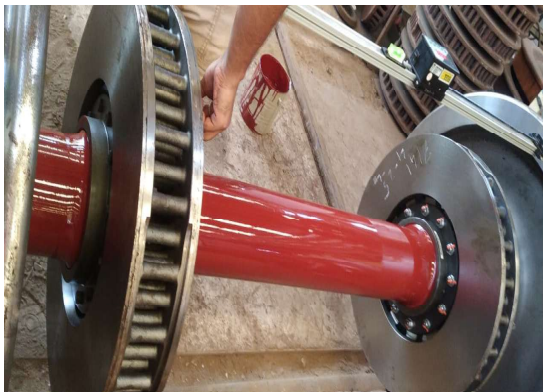
Primer Coated of LHB Axle body
