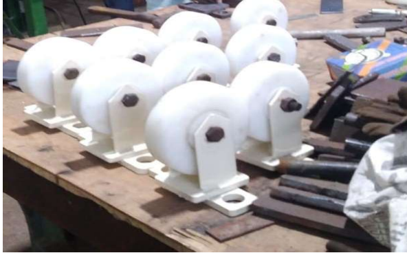
Finished supporting wheel fixtures of \
