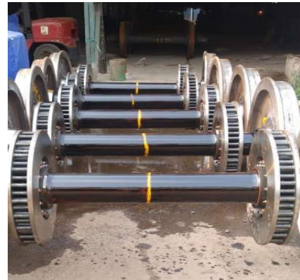
Finished LHB Axle body
