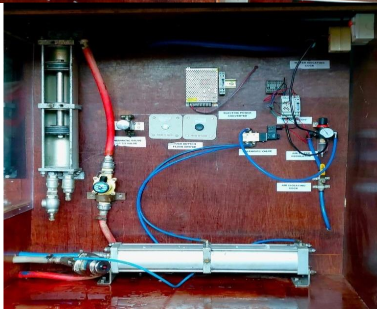
TEST BENCH OF PRESSURISED FLUSHING SYSTEM(PFS & EPFS) AT NCC/SDAH
