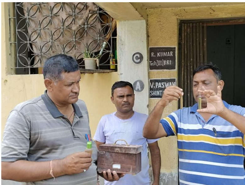
Residual Chlorine water testing at Rly. Colony, Sitarampur
