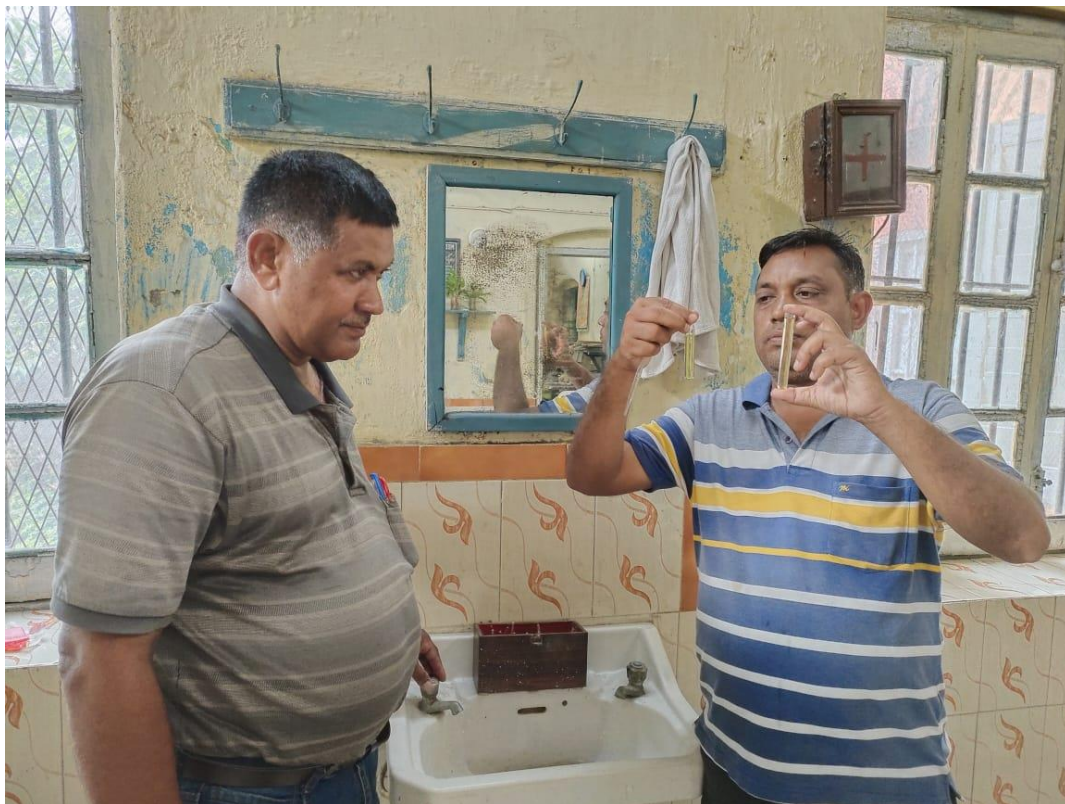
Residual Chlorine water testing, Health Unit, Sitarampur
