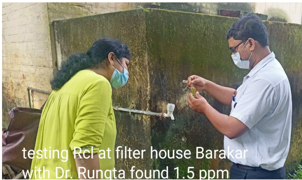
Inspection of water sample for chlorination at Filter house Barakar
