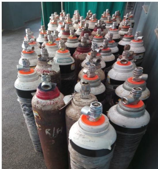
Oxygen Cylinders ready for refilling
