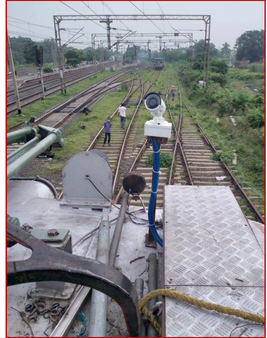
CCTV Camera Installed on Roof of Tower Wagon
