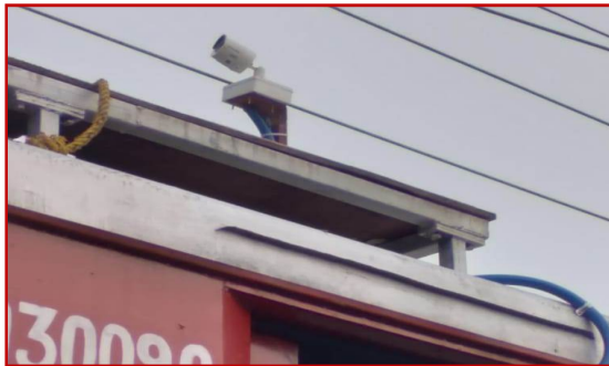
CCTV Camera Installed on Roof of Tower Wagon
