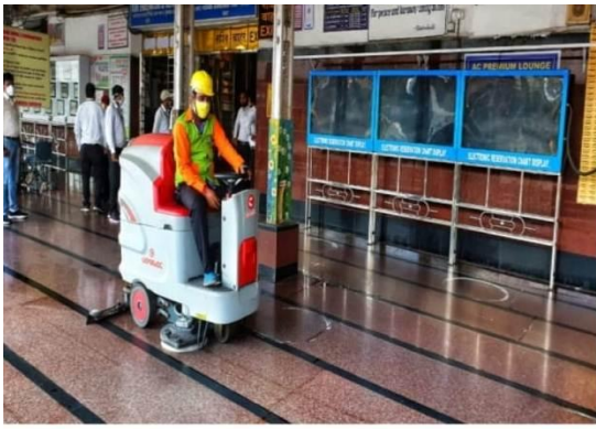
Cleaning with Scrubber drier machine at Asansol Station on 17.09.2020
