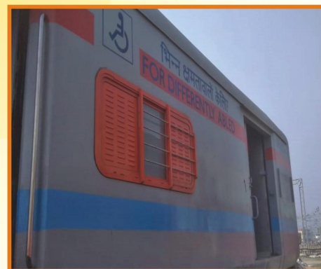
Newly Manufactured LHB Power Car with Compartment for Differently Abled Passengers
