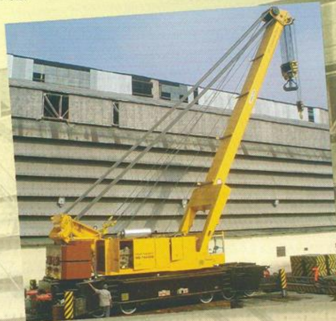
140T Gotwald design Break down crane manufactured by JMP
