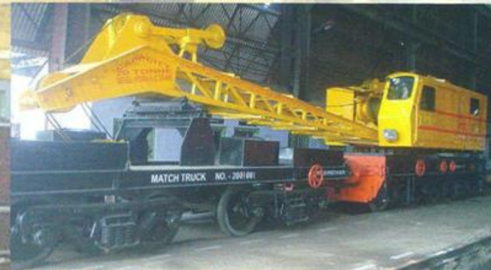
20T Diesel crane manufactured by JMP
