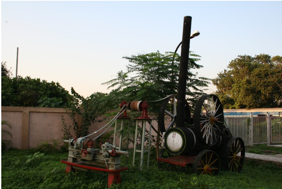
Steam engine driven lathe machine
