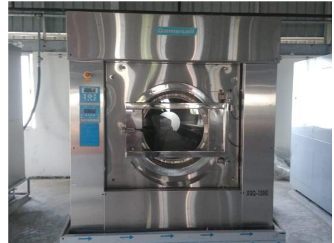
Industrial Big Washer Extractor for Bed Sheet
