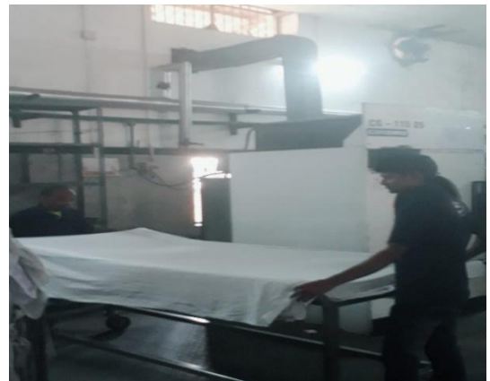
Stretching of Linen before calendaring
