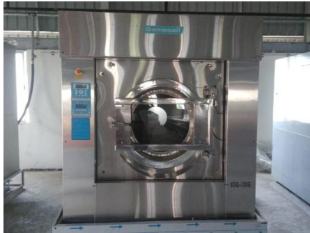
Industrial Big Washer Extractor for Bed Sheet
