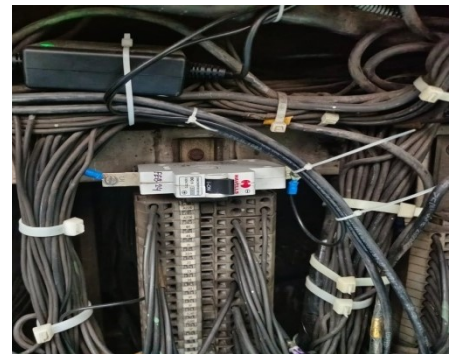
01 Amps MCB provided under Driver's Desk for safety of the equipment
