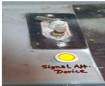
Signal Approaching Device Acknowledgement Switch provided on Driver's Side in front of Wiper Operating Switch for easy access of Driver
