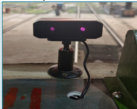
AI Camera to track Driver Eye Movement & Detect abnormal Blinking patterns
