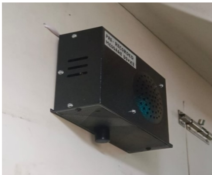
Signal Approaching Device installed on roof cabinet above Driver's position for clear hearing of the alert message
