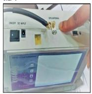
INSERT THE GPS ANTENNA PIN GENTLY, PLACE ANOTHER END OFGPSCABLEAS MUCHASOUTER SIDE OF LOCO.
